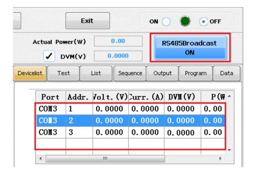
Monitoring software of this series power source add global control function. With RS485 communication, it is available to connect 30 units of different models and there are two ways to set output parameters:
